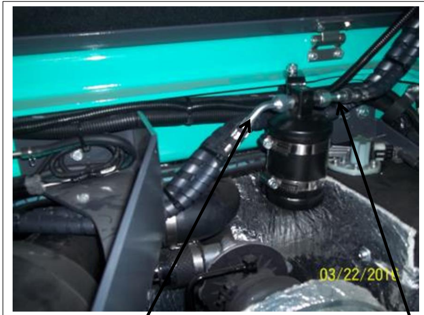
#6 45° fitting to expansion valve
