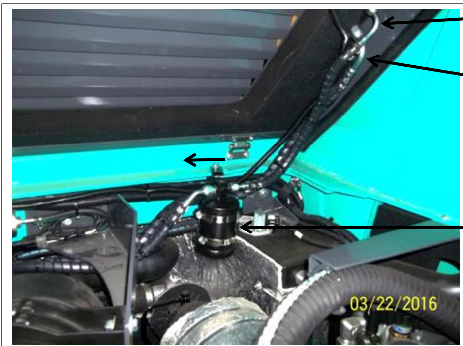
90° drier bracket mounts here in engine compartment. Right side near hood hinge.
