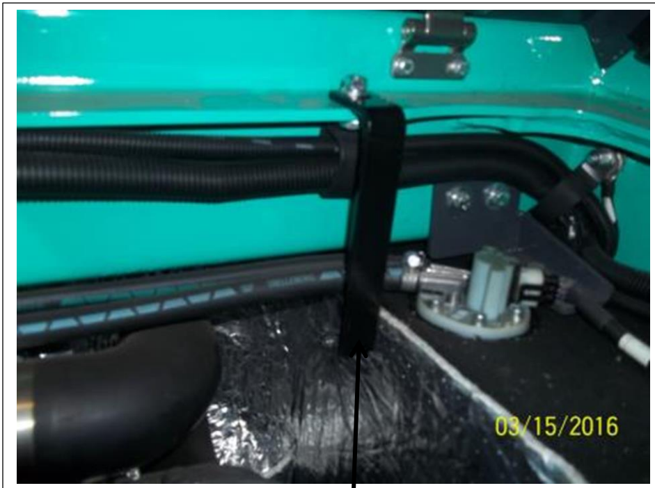
90° drier bracket mounts here in engine compartment. Right side near hood hinge.
