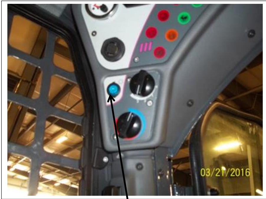
AC on/off switch added
