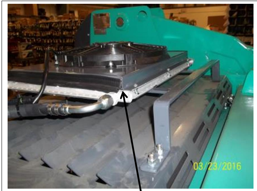
Condenser assembly installed on engine cover
