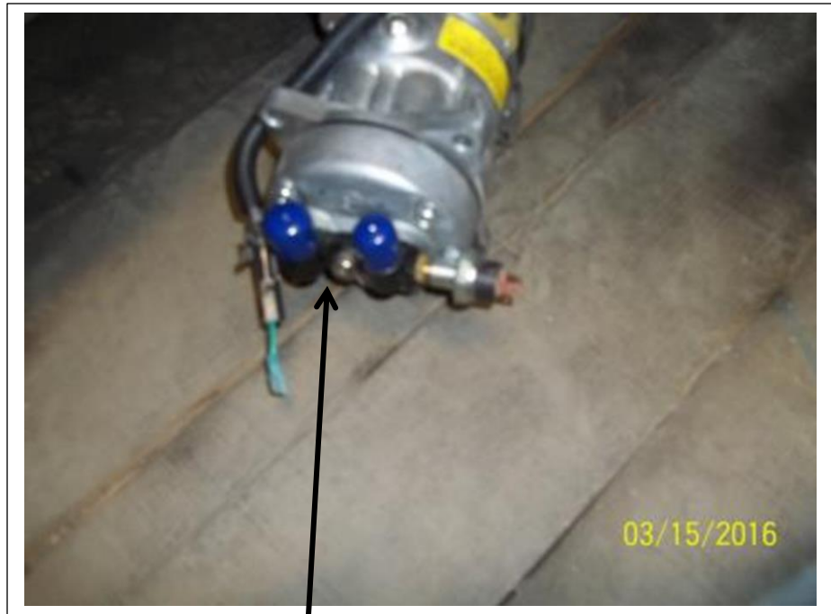
Install pad onto compressor
