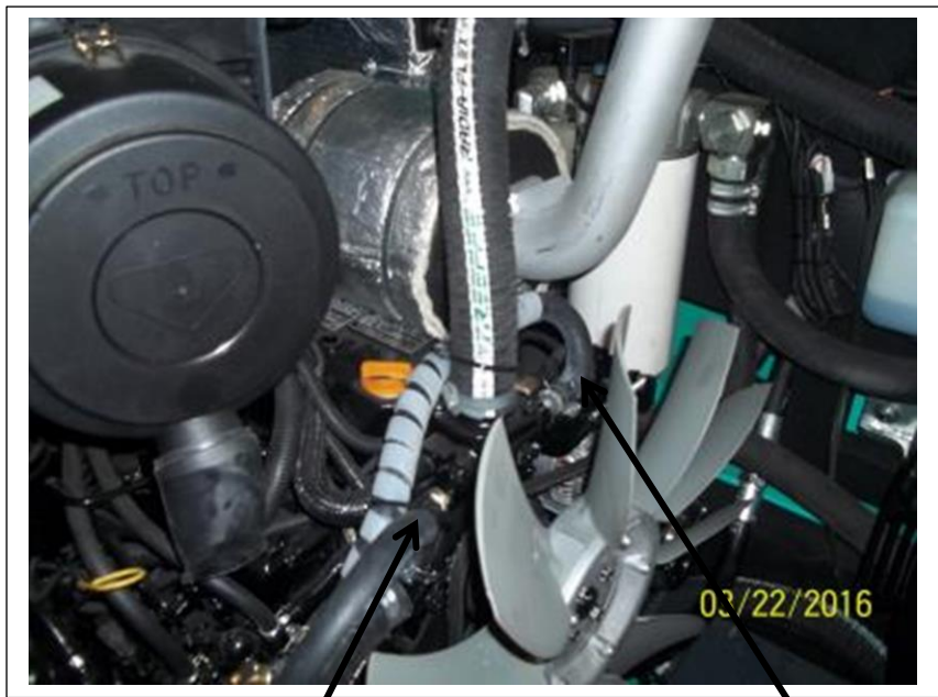
Return line for heat goes here. Remove plug and install fitting with hose barb.
